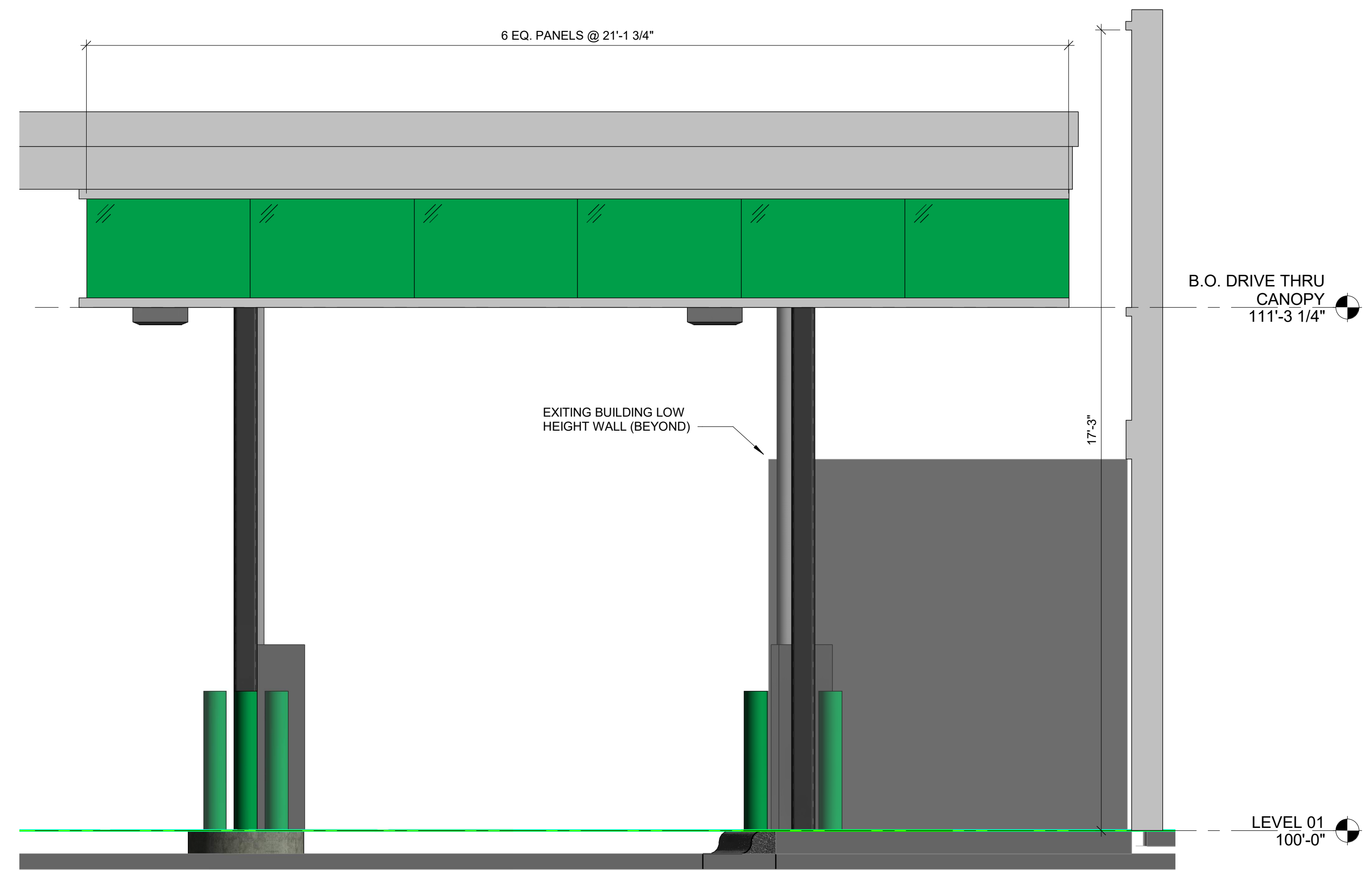
3 EAST ELEVATION - DRIVE THRU CANOPY 1/2" = 1'-0"
