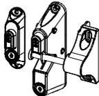
Locking Gravity Latch with 2-sided Key Entry/Push Button
