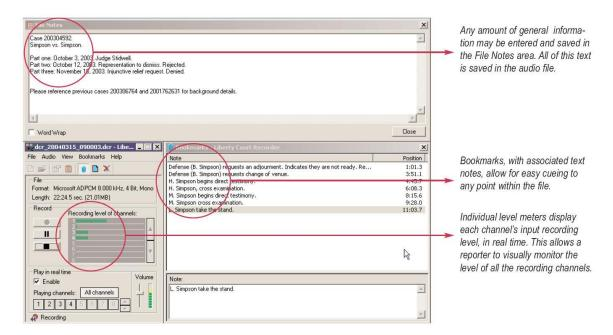
The **Player** is also intuitive and simple to use. With the Player software the user can control the playback of the audio and copy recorded audio. The Player runs on any PC with Windows 98 or later and uses the PC's standard sound card.
