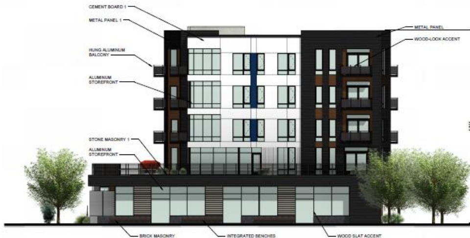
View of northern building looking west from recreation area adjacent to the proposed development (see attachments for full renderings with ability to zoom in on details).
