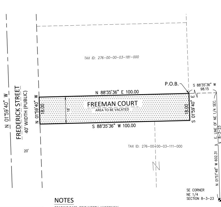
BEARING BASE: GRID NORTH, WISCONSIN COORDINATE SYSTEM, SOUTH ZONE. BASED UPON NAD 1983 / 2011.
