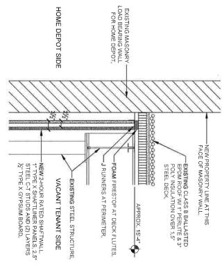
NOTE: EXISTING SUSPENDED CEILING TO BE REMOVED AS NEEDED & EXISTING STUD WALL TO BE REMOVED, UPON INSTALLATION OF NEW SHAFTWALL EXISTING COLUMNS TO BE STUD & DRYWALL WRAPPED AND SUSPENDED CEILING RE-FITTED.
