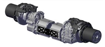
Communities with more demanding conditions and tougher terrain may opt for the DuoPower™ drivetrain, which provides unparalleled performance and up to 25 MPGe. Featuring two electric motors, this drivetrain can accelerate the ZX5 1.5 times faster than a standard diesel bus, with nearly twice the horsepower, enabling industry-leading hill climb capabilities.
