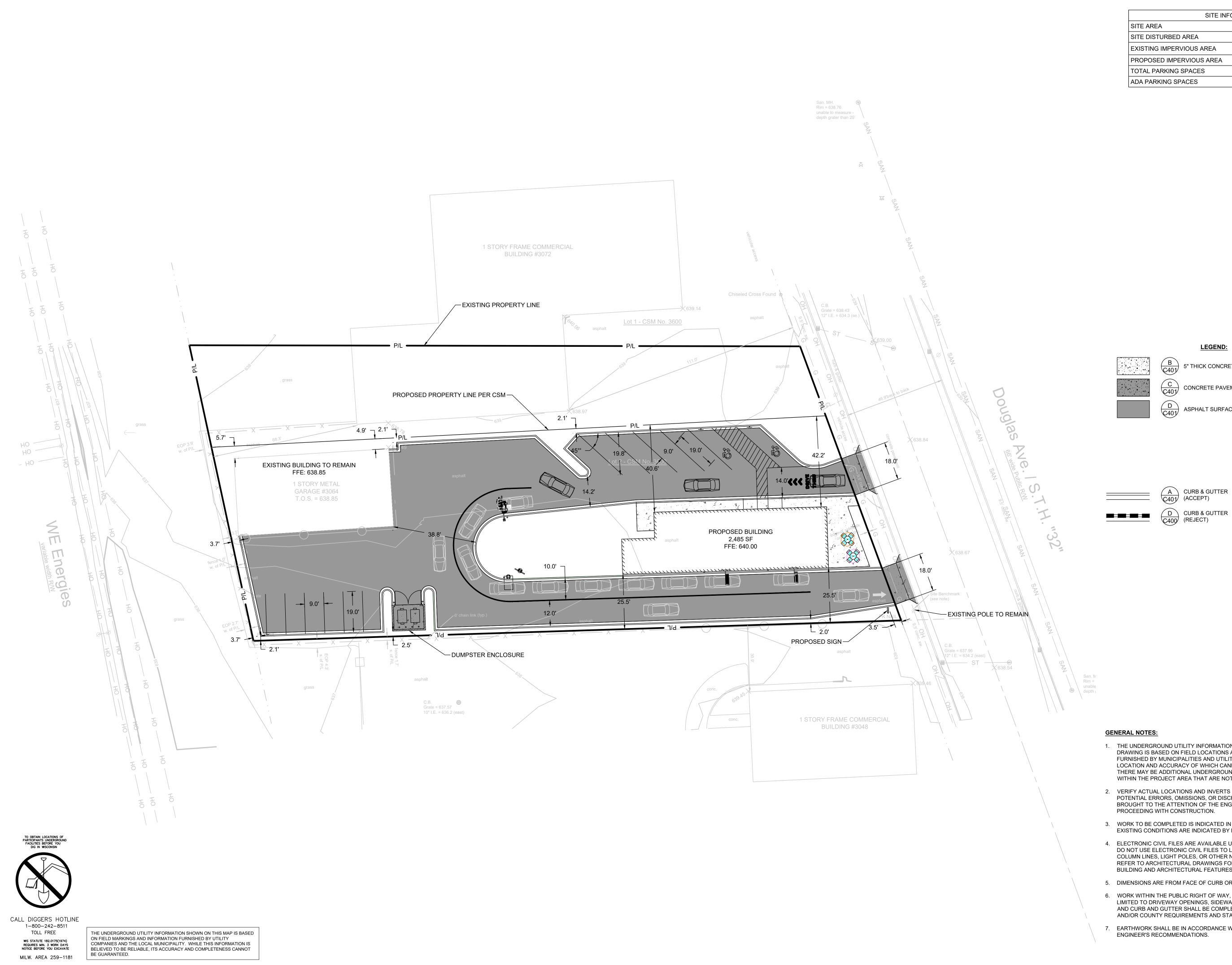
SITE INFORMATION 27428 0.630 AC SITE DISTURBED AREA 25087 0.576 AC EXISTING IMPERVIOUS AREA 27428 0.630 AC | 100.0 % PROPOSED IMPERVIOUS AREA 24055 0.552 AC 87.7 % TOTAL PARKING SPACES 13 ADA PARKING SPACES 2
