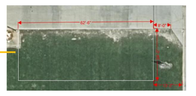
Shown above is the size of the new paved area to be added on the south end of the concrete lot. This pad will be sloped to the south into the grass.
