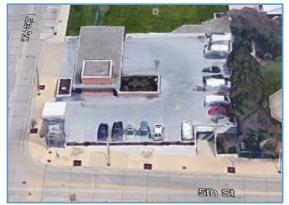
of the parking structure. It is our understanding that the bank building and teller lanes, with the exception of the ATM location will be demolished in the near future. In addition, the large planter box will be lowered. These modifications are intended to reduce the overall loading of the structural support system.
