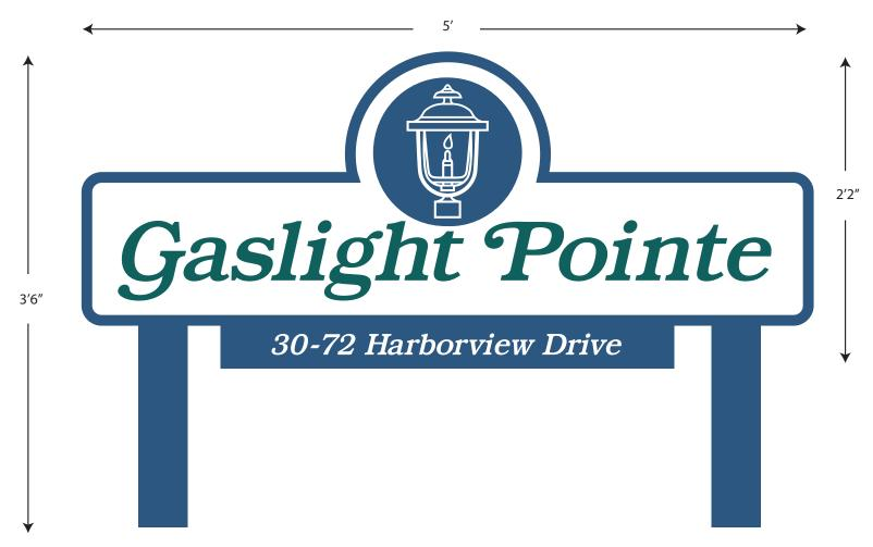
(1) Single-sided, high density polyurethane foam sign, sandblasted, with woodgrain finished background, mounted on 4" x 4" posts embedded in concrete. One LED light fixture will be installed in-ground in front of sign to provide illumination. For Owner: Gaslight Pointe Association, 120 E Chestnut St., Burlington, WI 53105, 262-661-4284, email carissa@mpcpm.com Date of drawing: 8.1.2019
