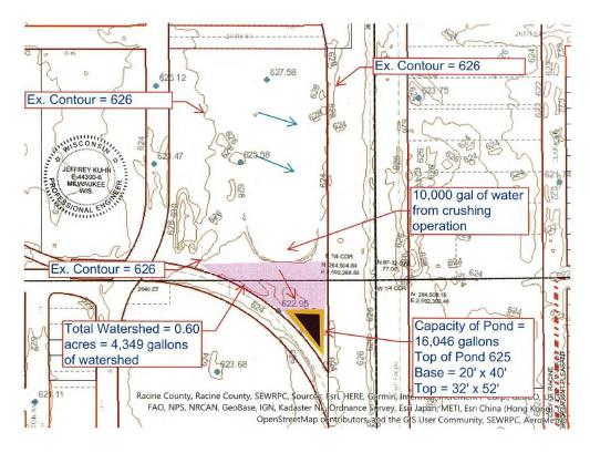
Site Plan with Contours indicating drainage towards retention pond.
